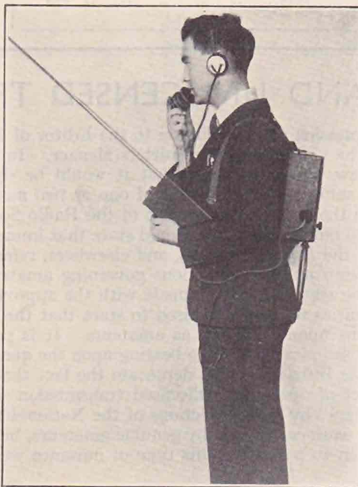
The complete station as worn when taking field strength measurements. Duplex telephony is used by the authors on these occasions.
